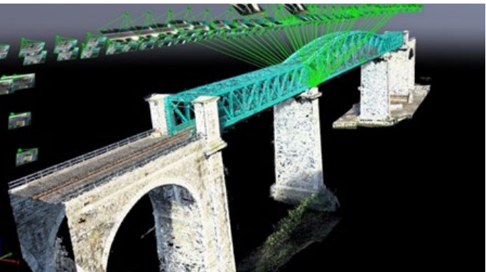
Figure: Point cloud data and inspection points during a drone survey of the Boyne Viaduct
