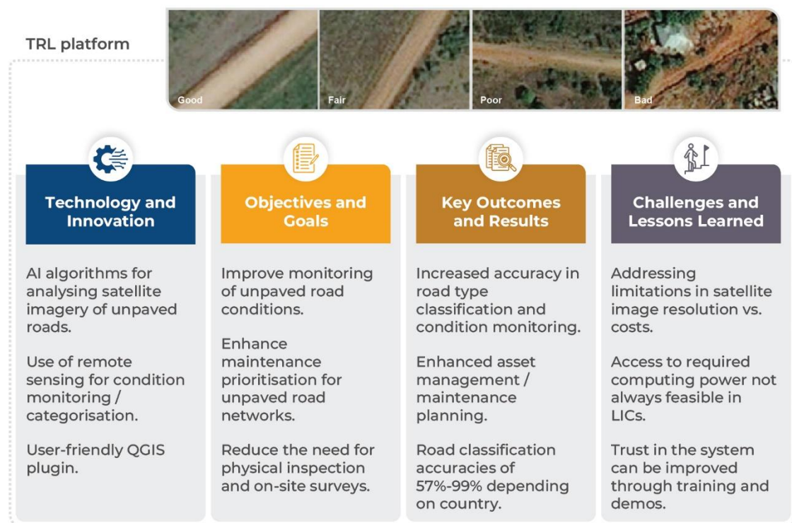
Figure 16: TRL - Monitoring of unpaved road conditions in Africa using satellite imagery and AI.
