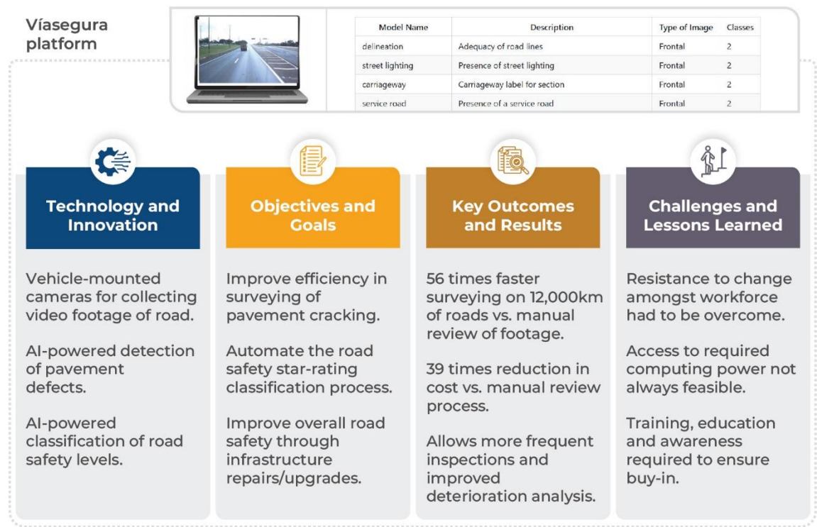
Figure 17: Víasegura - Automated classification of road safety and pavement condition in South America.
