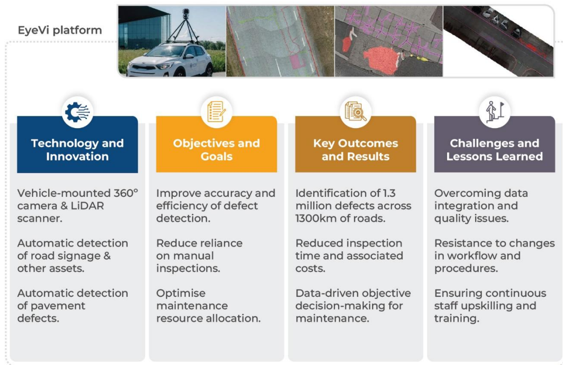
Figure 11: EyeVi platform - digitalisation of defects on Oslo's urban road network
